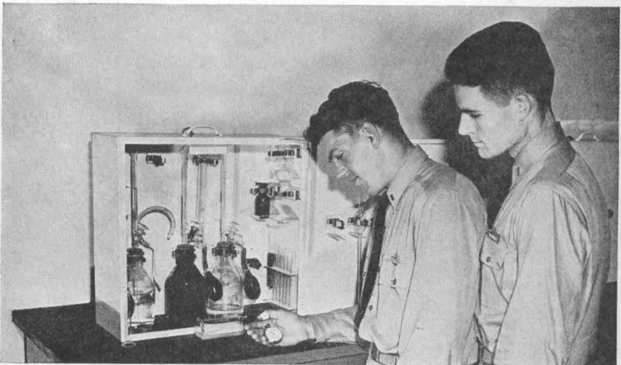
Student Navy Officers Run Boiler Water Test
