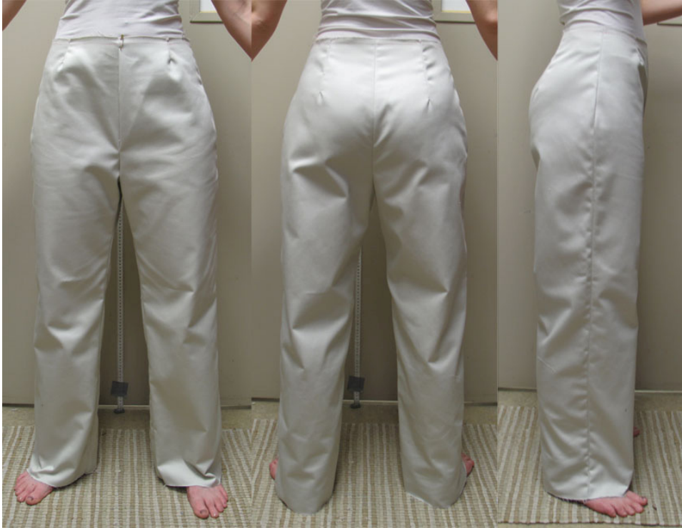
Figure 4-20. #79 (the final fit model) - group 3. The inseam length was shortened by 0.6 cm (0.25 in). The side seam was moved toward the back by 0.6 cm (0.25 in).
