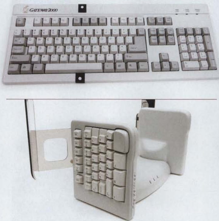
The conventional flat keyboard (top) and an experimental split version, which allows users to type in a more natural, relaxed position.
