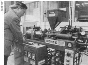
▲ Prof. K. K. Wang, mechanical and aerospace engineering, adjusts the plastic injection molding machine, which pumps liquid plastic into a specific mold. Wang has developed a sophisticated computer program that will simulate the molding process before it is done on the factory floor, eliminating the costly process of trial and error.
