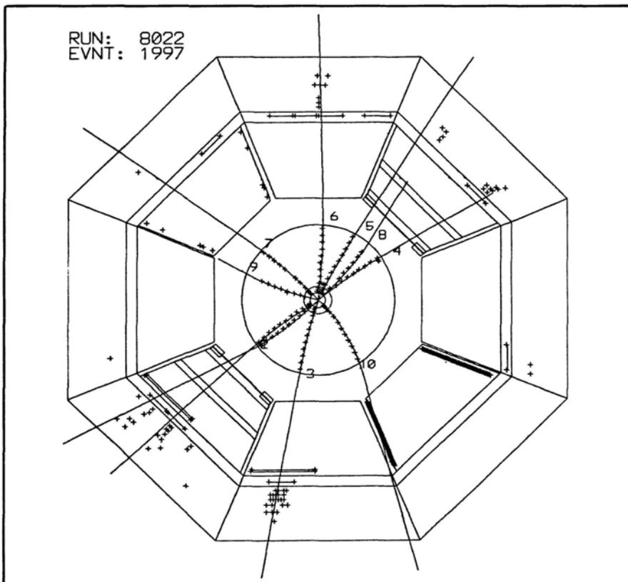
This drawing represents the products of a collision of electrons and positrons in the 'Cleo' detector of the Cornell Electron Storage Ring, CESR, in June 1980. Beams stream in and out of the plane represented by the page, collide head on, and annihilate each other. Their energy rematerializes in the form of a particle known as an *upsilon meson*. The numbered tracks correspond to the charged particles that arise from its decay. The center region corresponds to the draft
