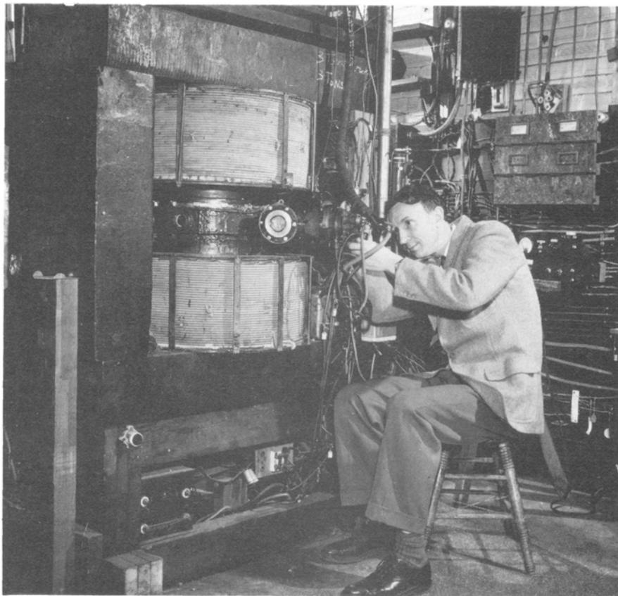
*In 1954 in the basement of Rockefeller, Prof. Boyce McDaniel peers into the university’s first particle accelerator, used from 1935-56. The cyclotron whirled protons around an orbit of 16-inch diameter at 1.5 million electron volts, MeV.*
