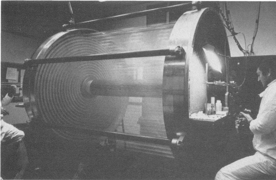
Drift chamber is prepared for the present Cornell particle accelerator. Particles will collide at the center of
