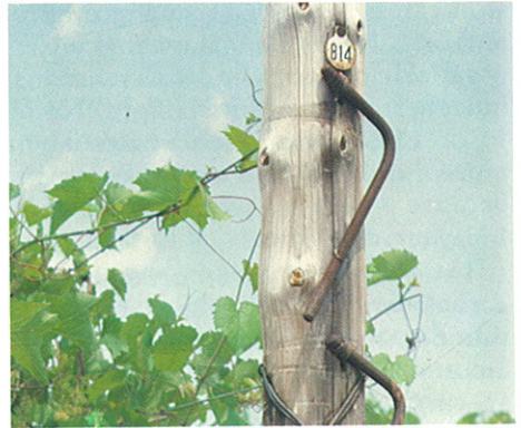
Figure 9. L-shaped cranks made from ½-inch steel rods provide a simple, rapid method to tension wires.
