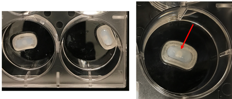
Figure 4.5. Photographs of composite TE-IVDs cultured in cages between media changes. Scale bars represent 17.5 mm while the red arrow indicates the location of the NP within the construct.
