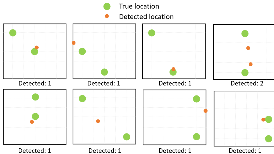
Figure 5.28 OMP grid results for two occupants showing true and detected locations. With two occupants, reflection model alone is very noisy.
