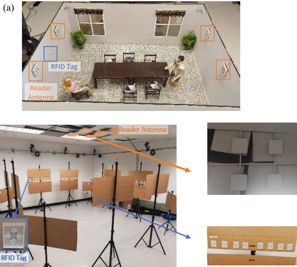
Figure 5.9 Experimental setups for occupancy monitoring with COTS RFID system. (a) A 1/6 th scaled model of a conference room setup with four small patch reader antennas on the four walls and RFID tags under the wallpaper. (b) The room scale setup with RFID tags on the cardboard and reader antennas on the ceiling, also shown in the zoomed insets.
