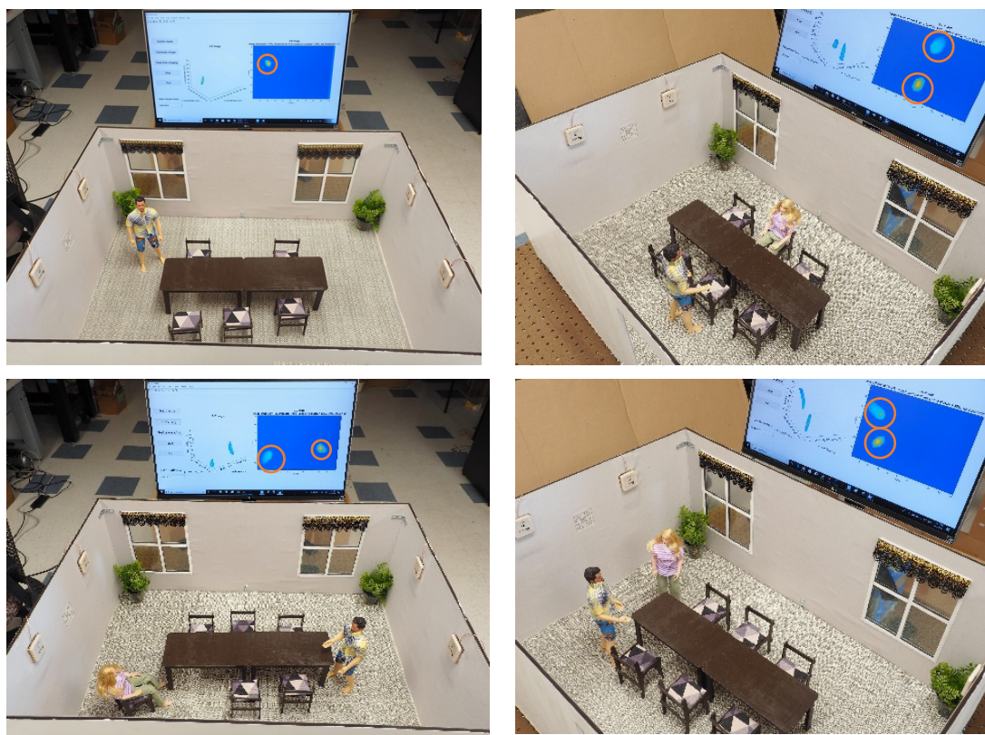
Figure 5.21 The scaled experiment setups with different object count, locations and postures, and corresponding generated images on the monitor, marked by orange circles.
