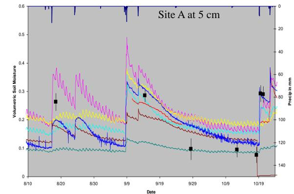
A comparison of the sensors at a depth of 5cm. There are dramatic variations in sensor response, but these are un-calibrated and improvement is expected when calibrations are completed in the spring of 2011. Validation samples are plotted with standard deviations
