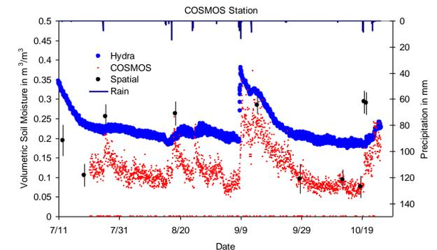
Early results of the co-located Climate Reference Network Hydra probe installation.
