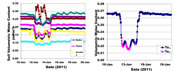
A comparison of different sensors and how they perform near 0 degree C. Unusual activity occurs prior to 0, which means a high resolution time series is important for accurate monitoring.
