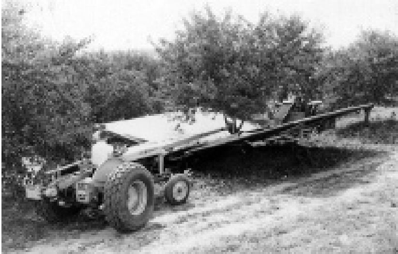
Cherry harvester: Tractor-mounted boom shaker and fruit-catching frame, with conveyor loader to the right. Harvesting time takes about 4 seconds.
