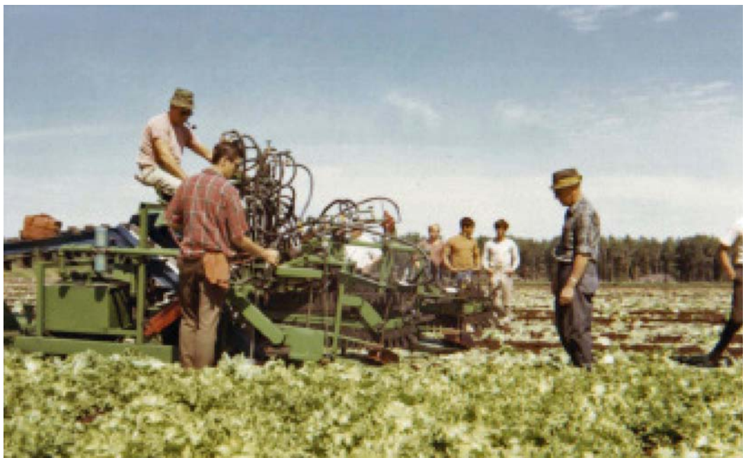
Field testing a prototype lettuce harvester. Professor E. Stanley Shepardson inspects the cutter head. A superbly equipped machine shop in Riley-Robb Hall makes new machine development like this possible, but places high demands on the personnel that resulted from a surge in faculty research activity.
