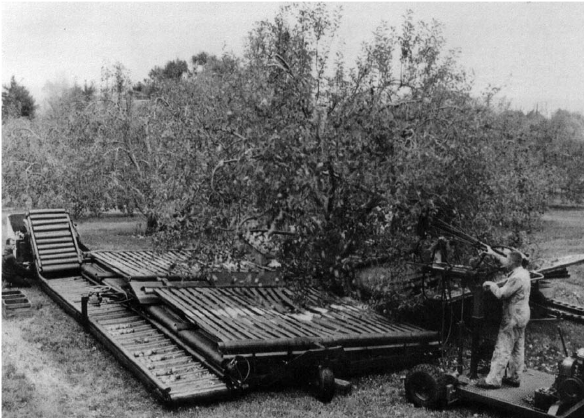
A 1965 mechanical harvester for apples to be processed. Fruit detached by the mechanical shaker on the right falls onto decelerating strips, then are moved on padded conveyors to a tiltable bulk box filler located behind the elevating conveyor at the left center. The bulk box is inclined to reduce bruising of the fruit by decreasing the distance the fruit drops into the container.
