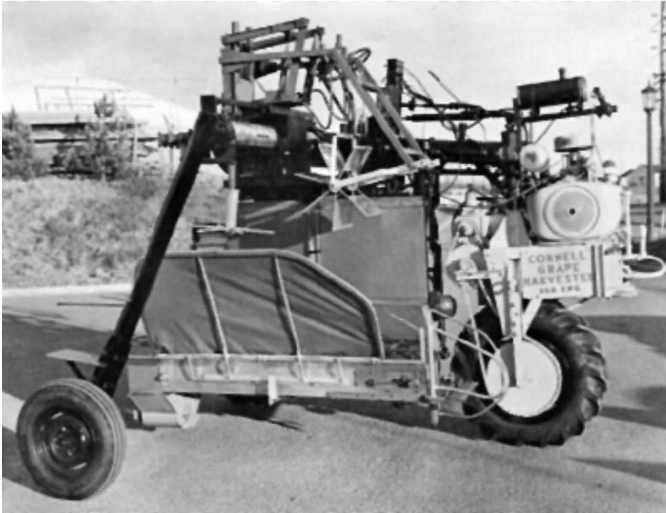
Final research version of the mechanical grape harvester in 1961.
