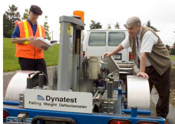
Dr. David Orr and Professor Lynne Irwin prepare for a falling- weight deflectometer roadbed test 50 years later in 2006.
