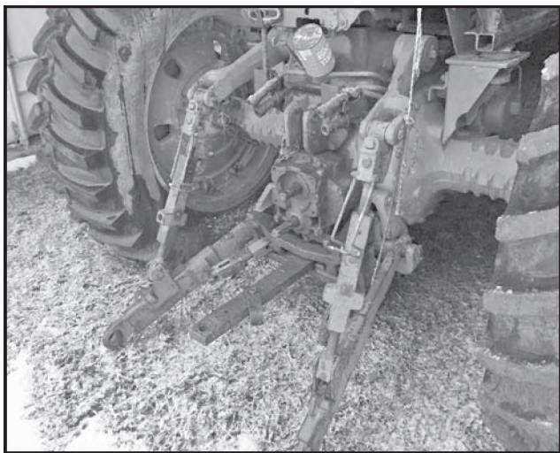
A typical fully functioning three point hitch
