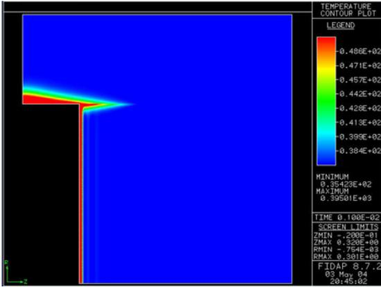
Figure 6: Temperature contour plot with conductivity value of  $0.2209 \times 10^{-6} \frac{W}{m \cdot K}$ .
