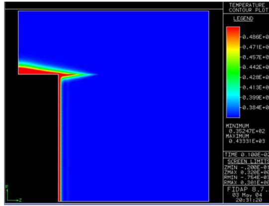
Figure 14: Temperature contour plot with density value of  $0.9 \times 10^{-6} \frac{kg}{cm^3}$ .
