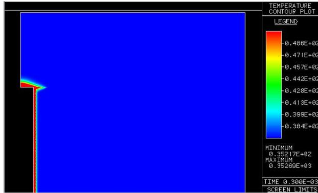
Figure 17: Temperature contour plot with laser power value of 9W.
