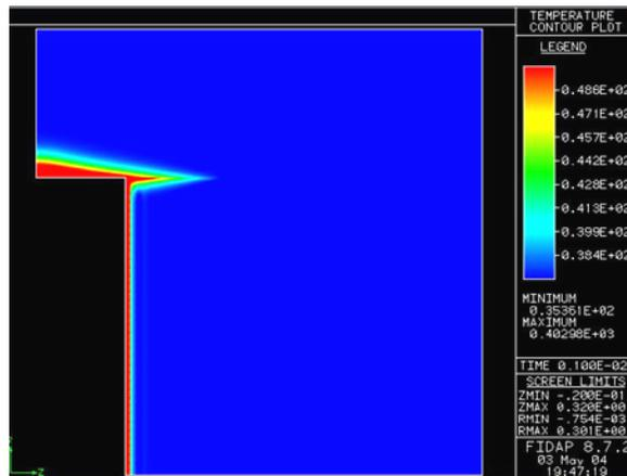
Figure 9: Temperature contour plot with convection value of  $5 \times 10^{-6} \frac{W}{mm^2k}$ .
