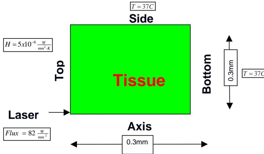
Figure 21: Schematic of the geometry with initial condition.
