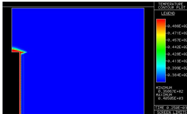
Figure 18: Temperature contour plot with laser power value of 12W.
