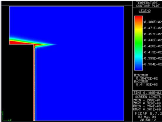
Figure 5: Temperature contour plot with conductivity value of  $0.1881 \times 10^{-3} \frac{W}{m \cdot K}$ .
