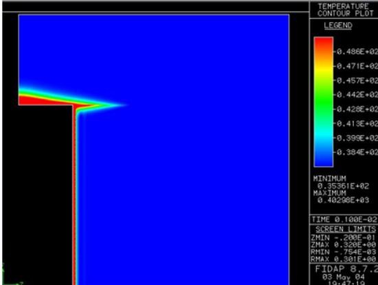
Figure 7: Temperature contour plot with conductivity value of  $0.2299 \times 10^{-6} \frac{W}{m \cdot K}$ .
