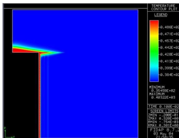
Figure 10: Temperature contour plot with convection value of  $50 \times 10^{-6} \frac{W}{mm^2k}$ .
