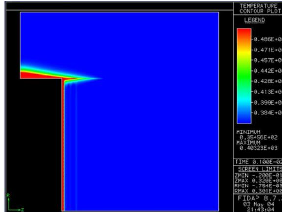
Figure 8: Temperature contour plot with convection value of  $25 \times 10^{-6} \frac{W}{mm^2k}$ .
