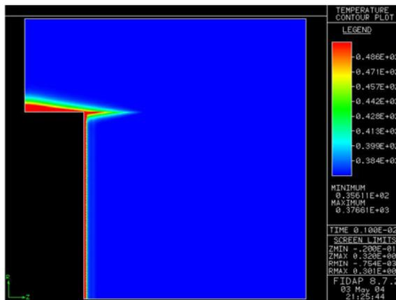
Figure 12: Temperature contour plot with specific heat value of  $4178.0 \frac{J}{g \cdot ^\circ C}$ .
