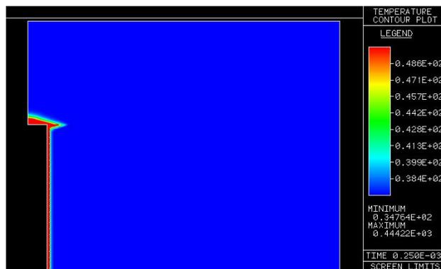
Figure 19: Temperature contour plot with laser power value of 15W.
