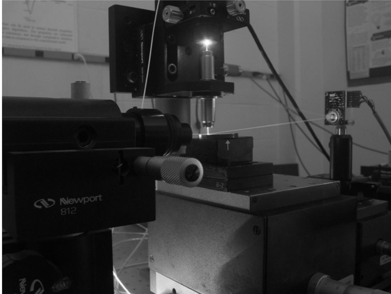
Figure 1: Photograph of PDS apparatus
