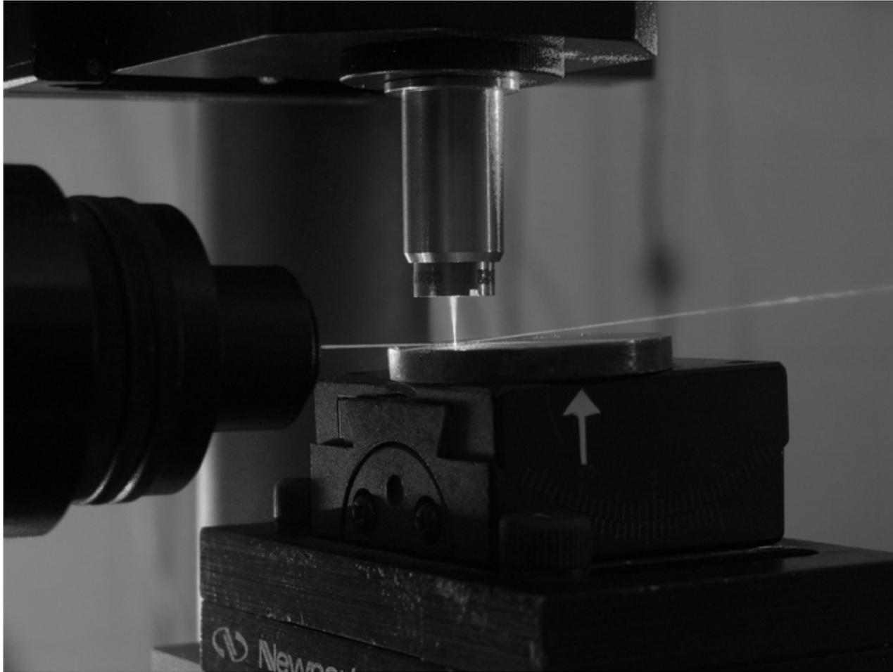
Figure 2: Heating beam and probe beam intersecting at sample surface
