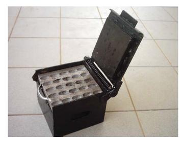
Fig. 1: A complete assembly of the village-level cashew nut sheller
