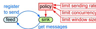
Figure 13. In our “pull” protocol stack a “feed” registers the intent to send with a “sink” that may be controlled by a policy limiting the send rate, concurrency etc. When the sink is “ready” to send, it calls the registered feeds for messages.
