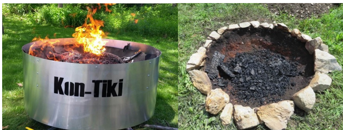
Figure 3: A metal flame curtain biochar kiln (left) and a soil pit flame curtain biochar kiln (right). (left: fingerlakesbiochar.com 2016, right: the biocharrevolution.com 2016). These kilns can be produced in various sizes and layouts.
