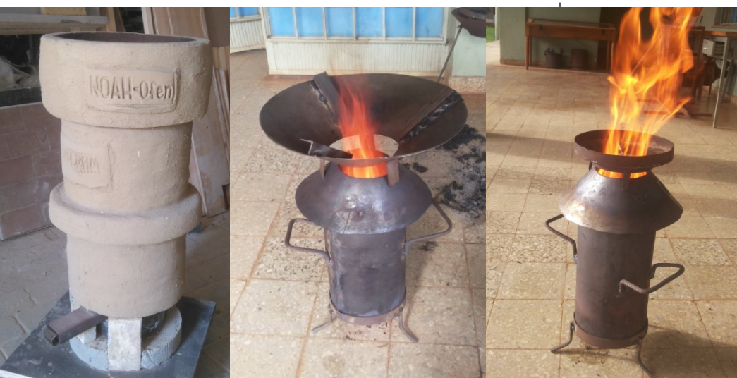
Figure 7: Pro Lehm Clay gasifier stoves (left) and Elsa metal gasifier stoves with different pot raiser (Venkata et al. 2016)
