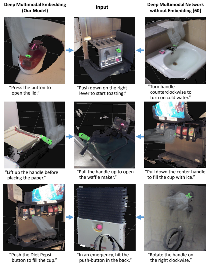
Figure 5.8: Comparisons of transfers between our model and the baseline (deep multimodal network without embedding [148]). In these three examples, our model successfully finds correct manipulation trajectory from these objects while the other one does not. Given the lever of the toaster, our algorithm finds similarly slanted part from the rice cooker while the other model finds completely irrelevant trajectory. For the opening action of waffle maker, trajectory for paper cutter is correctly identified while the other model transfers from a handle that has incompatible motion.
