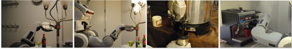
Figure 5.13: Examples of transferred trajectories being executed on PR2. On the left, PR2 is able to rotate the ‘knob’ to turn the lamp on. In the third snapshot, using two transferred trajectories, PR2 is able to hold the cup below the ‘nozzle’ and press the ‘lever’ of ‘coffee dispenser’. In the last example, PR2 is frothing milk by pulling down on the lever, and is able to prepare a cup of latte with many transferred trajectories.
