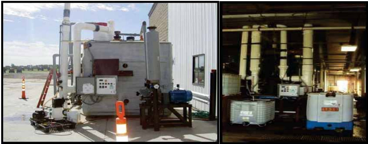
Figure 6: Batch testing of (a) aeration system and (b) two-tower acid contact system
