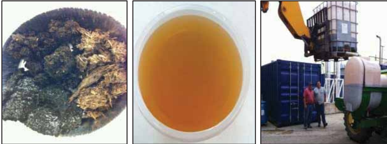
Figure 10: NR products: (A) three solids, P-solids, Fine-solids, Fiber-solids clockwise from left; (B) 35% solution of ammonium sulfate and (C) first application of ammonium sulfate to fields
