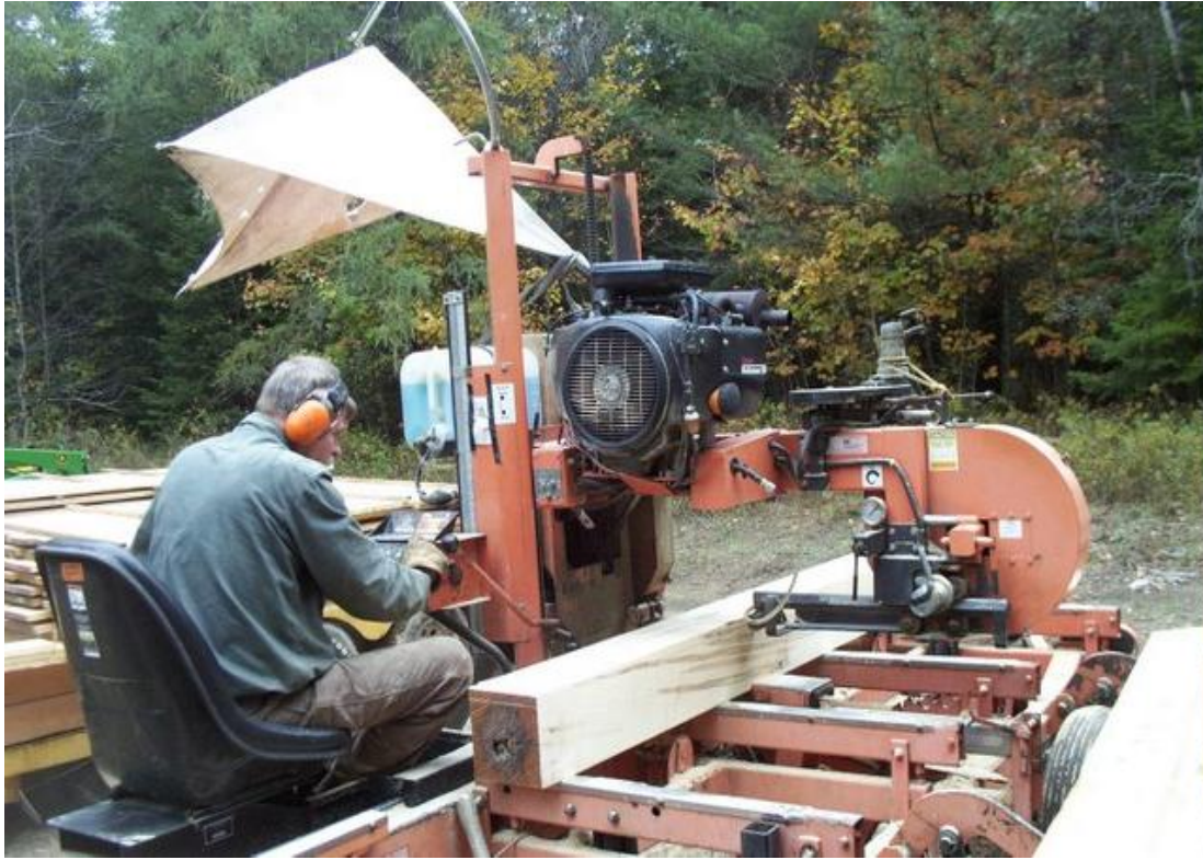
Figure 4.6 A tapped maple log being sawn into boards with a portable bandmill- note the prevalence of old tapholes and the associated stained columns.
