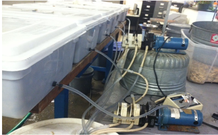
Figure 4. The image above shows the lab scale denitrifying bioreactors connected to the inflow feed tubes, which had their pump rates controlled by the blue pumps.
