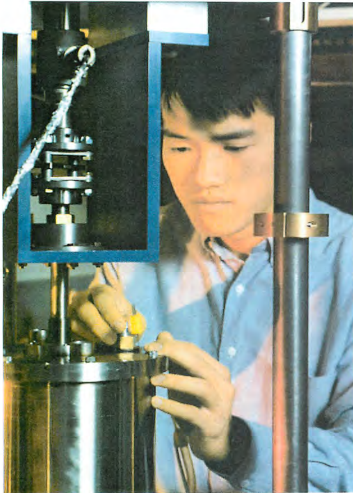
A specially designed apparatus is used to study the viscosity of semisolid metals.
