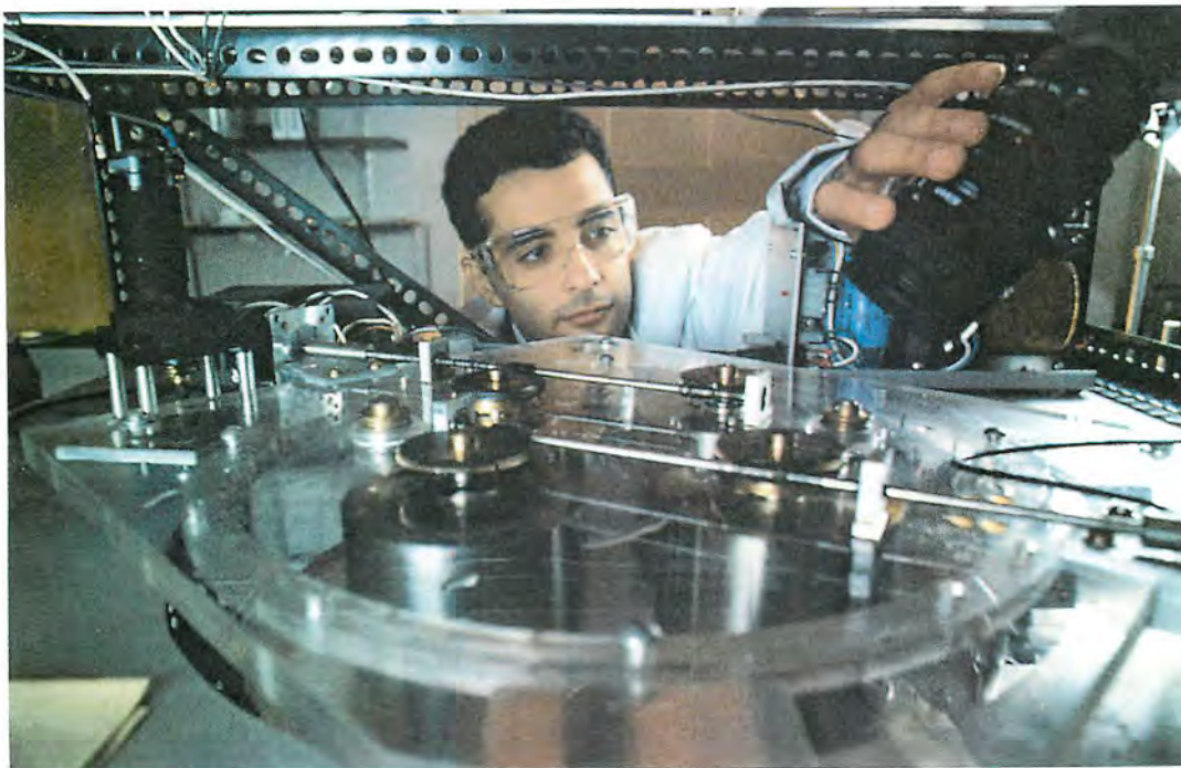
A four-roll mill is used to investigate the effect of polymer flow on fiber orientation.
