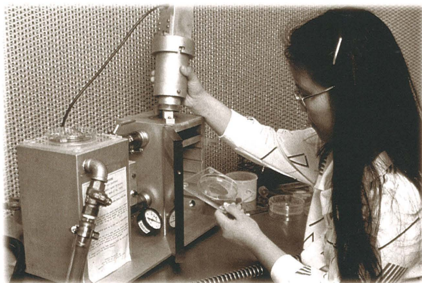
An early version of John Sanford's gene gun used to transfer genes from one plant to another.
