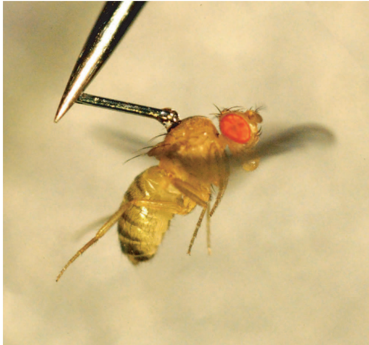
Figure 5.6: A common fruit fly ( D. melanogaster ) with ferromagnetic pin glued to the dorsal surface of its thorax is suspended by a magnetized sewing needle. The pin is 1.5 mm long. In free-flight, the insect is perturbed by application of a magnetic field that induces a torque on the pin.
