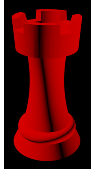
Figure A.1: The AMF file can use a simple list of vertices and triangles to define a mesh and replicate the functionality of an STL file, but without leaks. The XML-compliant format makes storing, parsing, and reading the file easy.
