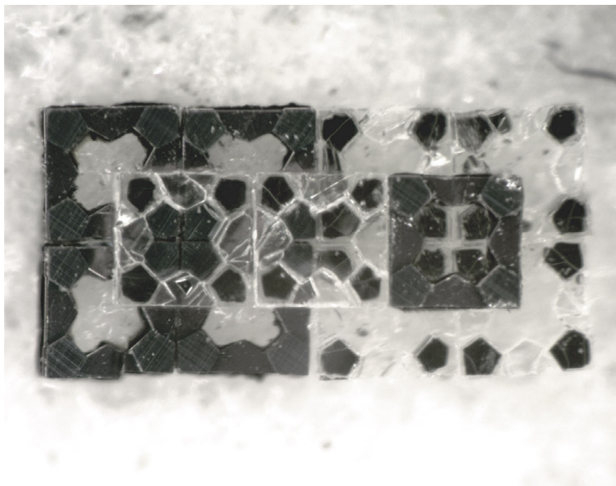
Figure 3.6: An 11 brick two layer multi-material structure was assembled by hand. Although the silicon bricks were too fragile to assemble on their own, combining them with the polymer bricks yielded a stable assembly. The dark tiles are silicon, while the translucent tiles are SU-8.
