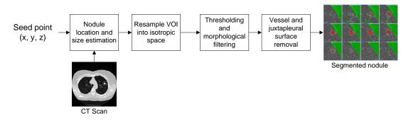
Figure 2.2: Flowchart of the pulmonary nodule segmentation algorithm
