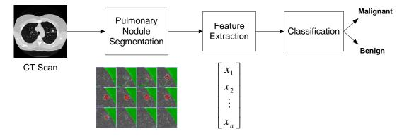
Figure 2.1: Overview of the nodule characterization system.
