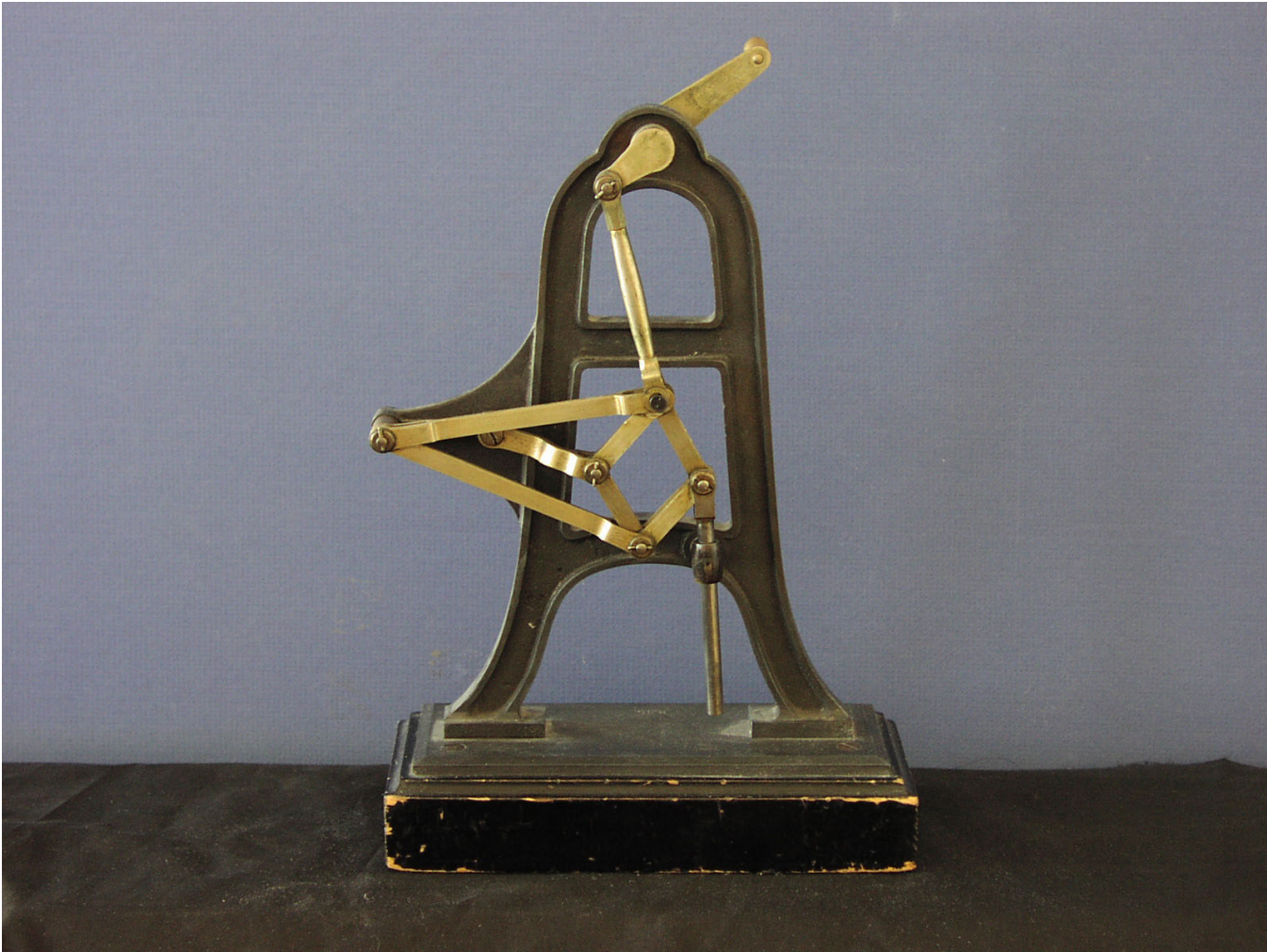
11. Peaucellier Straight Line Mechanism, c 1876. Model S35, Voigt Catalog, Cornell Reuleaux Collection.
