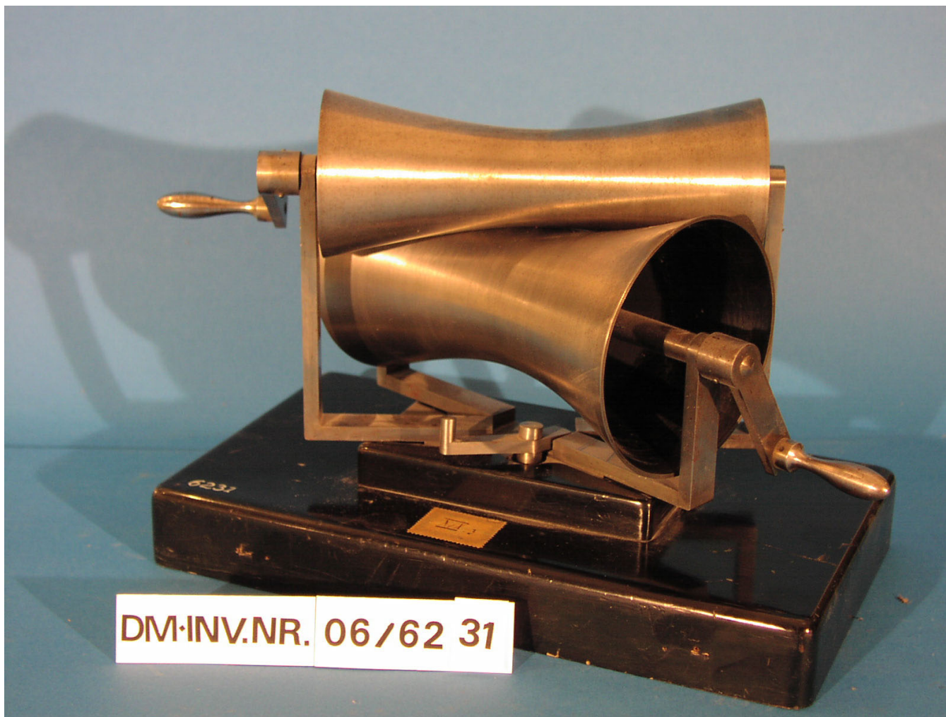
b) Rolling hyperboloid friction wheel mechanism. Model in the Deutsches Museum, Munich.
