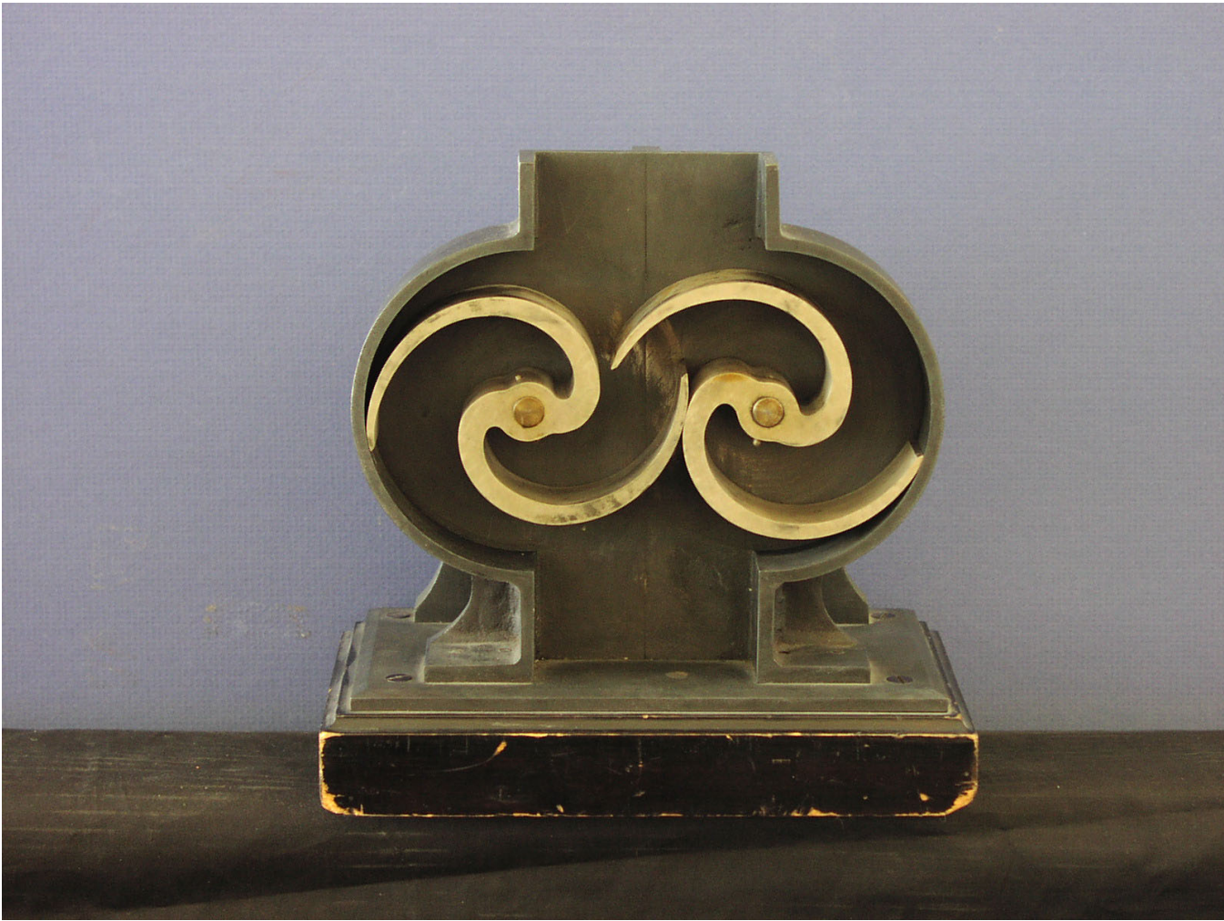
13. Chamber wheel train for a steam engine or pump. Model I4 Voigt Catalog, Cornell Reuleaux Collection.
