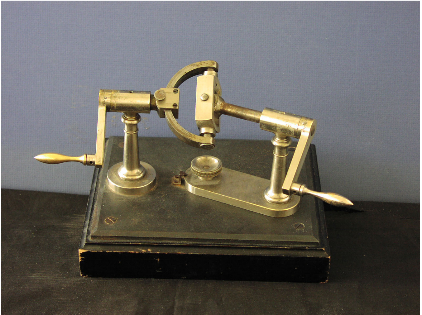
7 a) Universal joint (Hooke or Cardano). Model No P1, Voigt Catalog, Cornell Reuleaux Collection.
