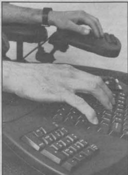
Adriana Rovers/University Photography A split floating arms keyboard (FAK) is mounted on the arms of a chair.
