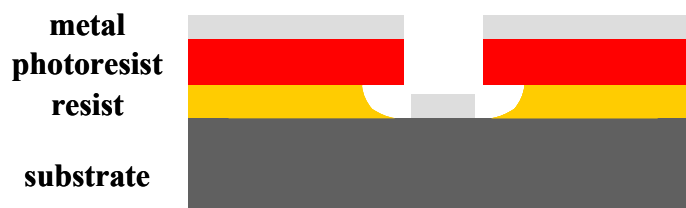
Figure 2.13 Schematics of metal lift-off process using a bi-layer resist process
