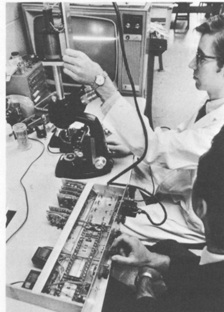
Shown here are two students of electrical engineering whose Master's thesis work requires the development of a video system to be used with a density-specific photometer. This device will aid researchers in differentiating and counting white blood cells. Their research is partially supported by the Virus Leukemia Research Grant of the New York State Veterinary College at Cornell.
