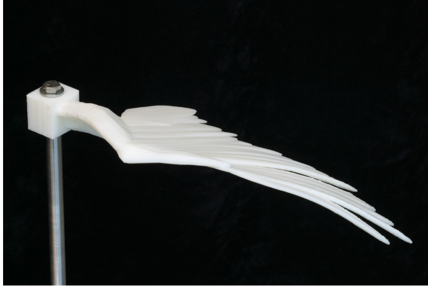
Figure 5.4: Plastic printed wing mounted on stand in wind tunnel for testing own insurmountable difficulties.
