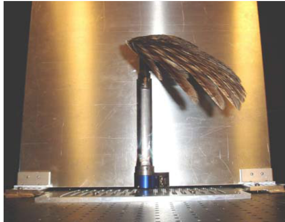
Figure 3.17: Red-tailed hawk wing with poseable wrist on a force transducer in a wind tunnel[MBG05]
