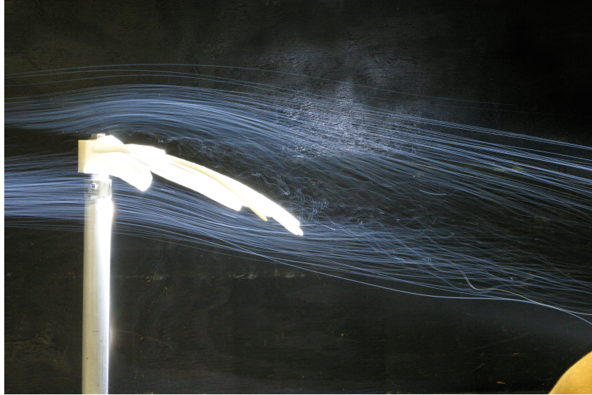
Figure 5.5: Plastic wing in wind tunnel with streaklines illuminated by helium bubbles
