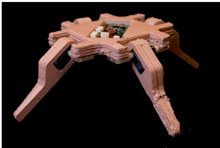
Figure 5.5. Robot after repair of its severed leg. (a) Top view. (b) Side view.
