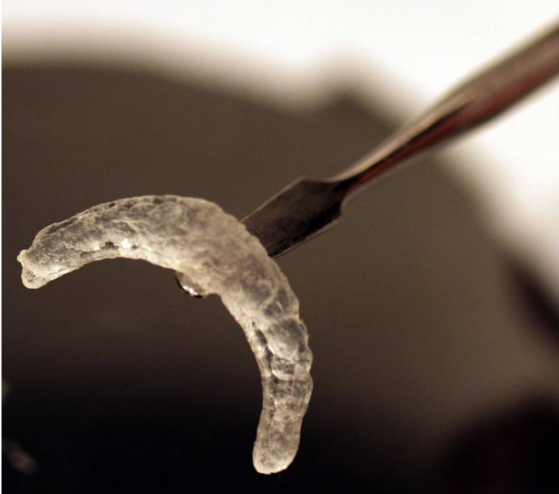
Figure 1.3. Printed crescent suspended with tool.
