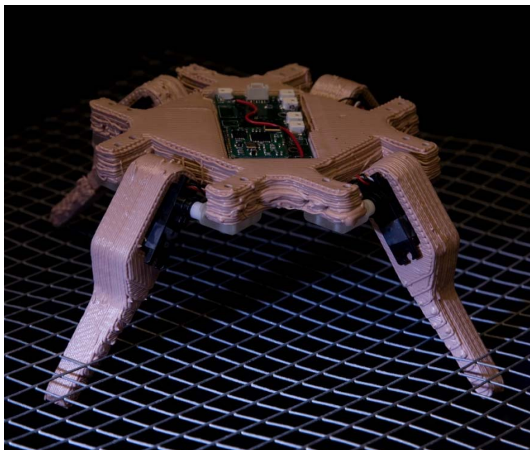
Figure 5.7. Prior to adaptation, the slender end of the robot leg slips through the mesh surface making traversal impossible.
