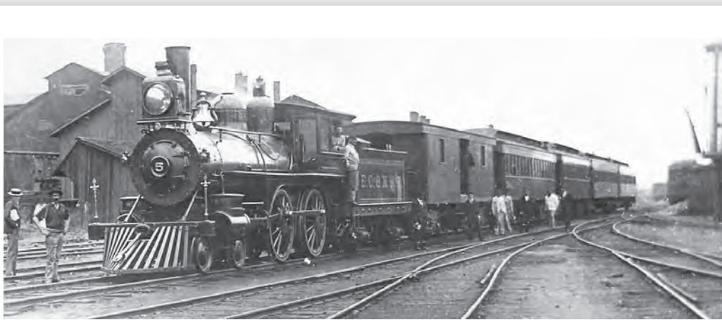
Engine 5 at Cortland Station with a southbound passenger train about 1889. According to the EC&N Book of Rules, as a southbound first-class train it has rights over all northbound and all inferior southbound trains.
