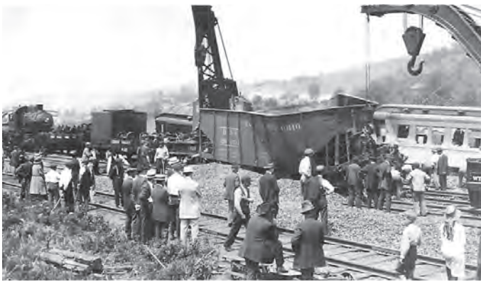
Wrecking cranes have uprighted the severely damaged fifth car of Extra 1155's train and prepare to remove it from Swamp Siding. The first and second cars of Train 6 are visible.
