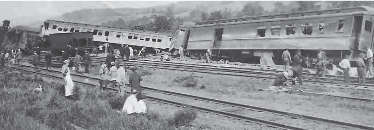
Bystanders and railroad personnel at the north end of the Van Etten yard after the May 1920 accident. Extra 1155 North with Engine 1162 assisting was traveling from left to right on the Swamp Siding when it derailed at the switch at the extreme right. Engine 2059 leading Passenger Train 6 traveled at 50 miles an hour from right to left and slammed into the tender of the freight train's lead Engine 1155 and into its second engine, 1162. From right to left are the fourth, third, second and first cars of Train 6 and two derailed hopper cars from Train 1155 North. BELOW: Train 6's Engine 2059 rests on its right side in the swampland, viewed from the Ithaca Branch main track.
