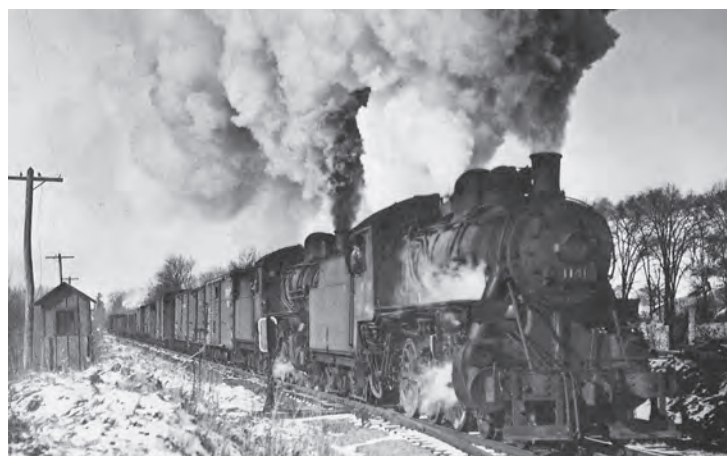
Two ten-wheelers on the headend and a third behind the caboose team up to move the northbound daily Cortland-Canastota freight at the south end of the East River passing siding on March 16, 1934. Note two telegraph wires near the center of the crossarm and a third telephone wire on the right side with connecting wire leading down to a telephone booth for crews to contact their dispatcher when necessary.
