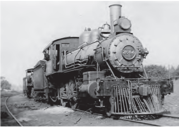
Engine 2644, a Class E-37 4-4-0, seen at Cortland about 1915, was built at LV Shops in Hazleton, Pennsylvania, in 1892 as LV Engine 644, rebuilt in 1916 and scrapped in 1924.
