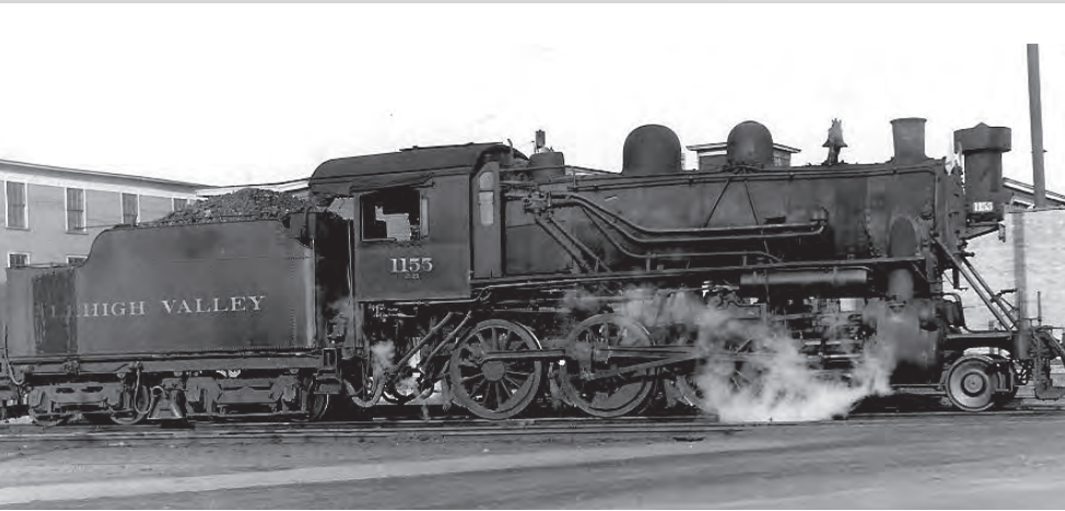
ABOVE: Engine 1155 was built by Lehigh Valley personnel at Sayre shops in 1918 as a class J-25 4-6-0, one of 35 such locomotives built by the LV in 1917 and 1918 for branch line duty. The J-25's were equipped with 63 inch drivers and weighed only 104,500 pounds on drivers. Engine 1155 saw regular service for over thirty years on the Elmira and Cortland Branch through the 1940's and was not scrapped until May 1950. It was involved in the May 1920 accident at Van Etten, discussed in the next chapter.
