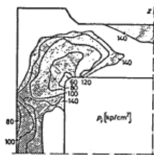
Circumferential Crack Zones
