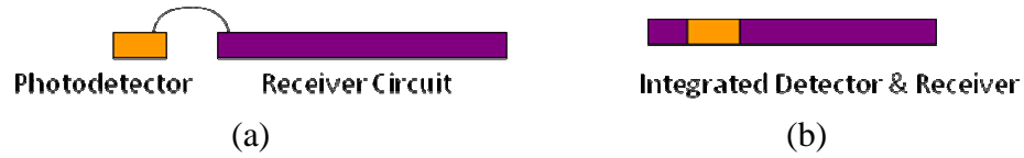
Figure 2.1 (a) Conventional detector integration, i.e. flex, wirebond, or flip-chip bond. (b) Monolithically integrated detector.
