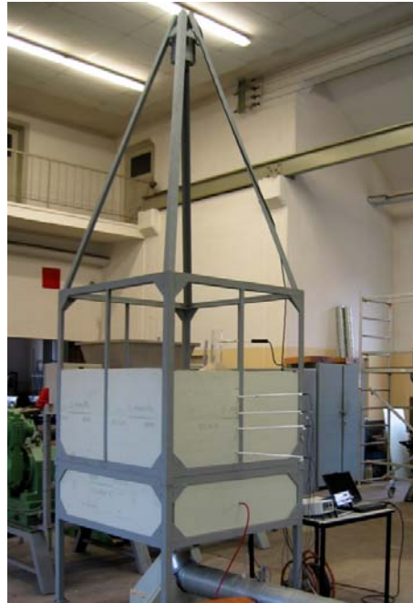
Figure 3: Ventilation test rig with square container, infrared thermographic camera in the rack tip
