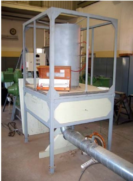
Figure 1. Ventilation test rig with cylindrical container
