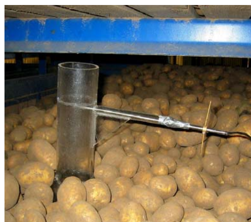
Figure 9. Measuring hopper with anemometer for measuring the air velocity
