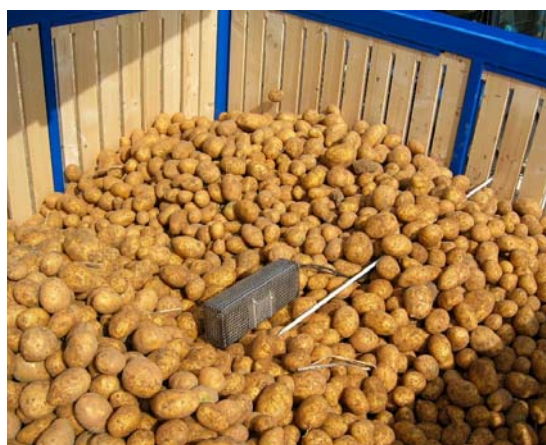
Figure 8. CO 2 gas sensor, temperature and moisture sensors in the middle of the box
