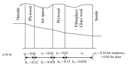
Figure 2. Construction of windows and door.
