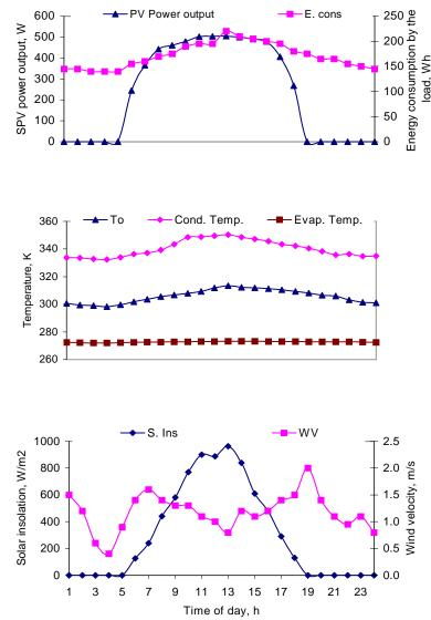
Figure 6. Effect of weather conditions on the SPV power output and energy consumption by vapour compression cooling system under full load during tested sunny days in summer 2001.
