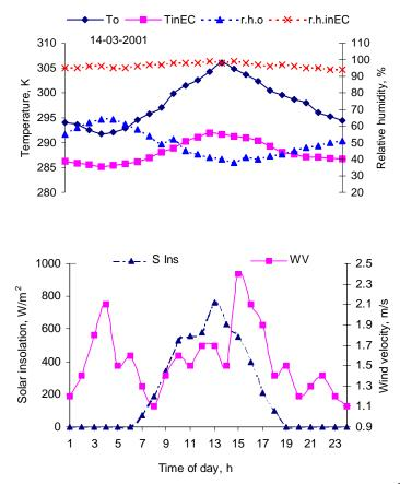
Figure 7. Effect of ambient conditions on the thermal environment in a 1m<sup>3</sup> empty EC structure with rice straw pad walls on a tested day (14-03-2001).
