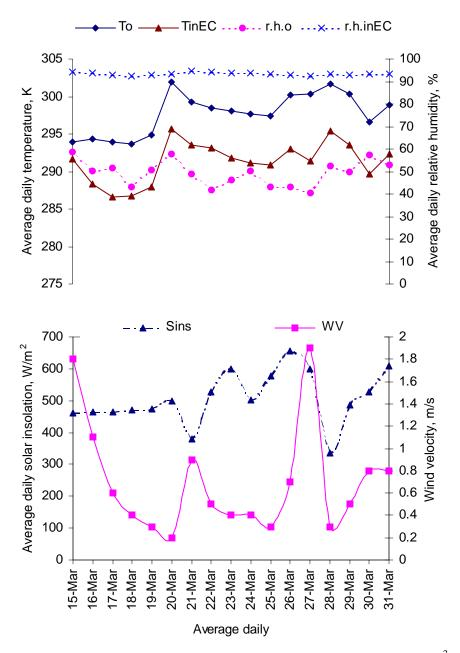
Figure 8. Effect of daily ambient conditions on thermal environment of 1.0 m<sup>3</sup> loaded EC structure during curing period (March 15-31, 2001).
