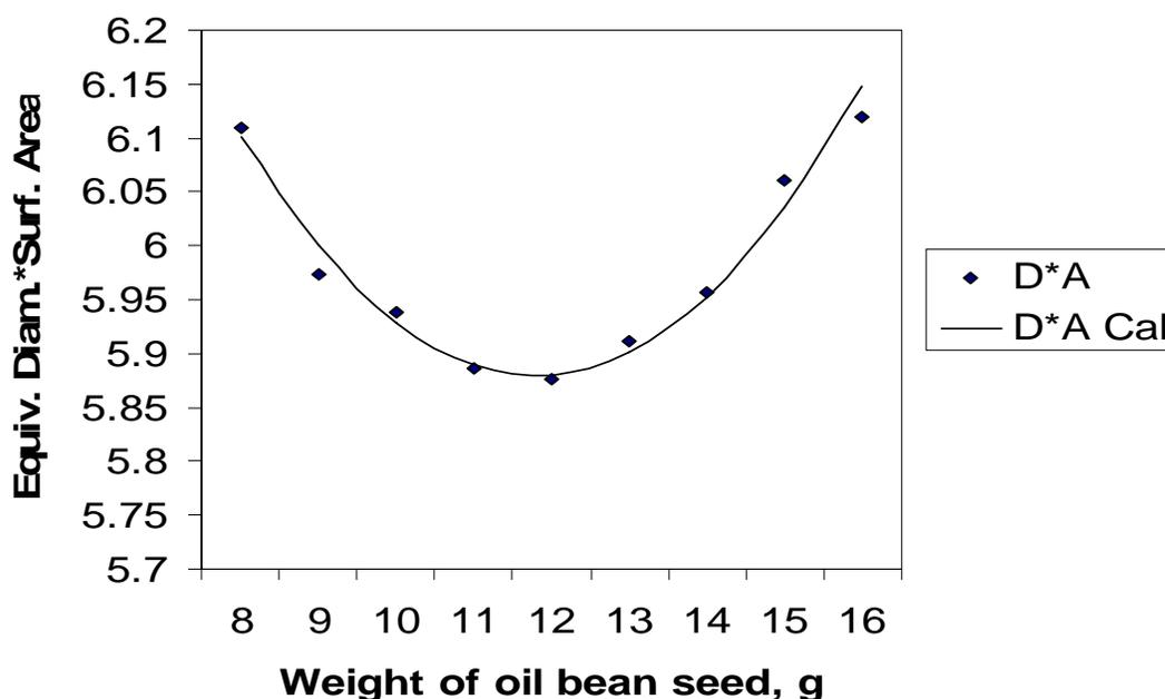
Fig. 2: Relationship between the product of equivalent diameter and surface area with seed weight
